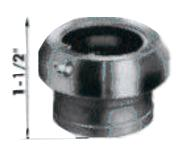
Our stuffing box uses double neoprene seals. Water must be discharged into the stuffing box, further lubricating the Aqua Lube bearing insert. O.D. is 1-3/4". For use with 1" and 1-1/8" shafts.
