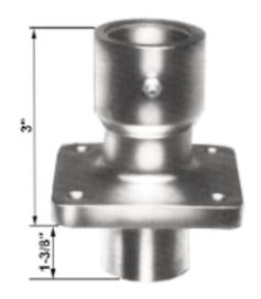
This competition rudder stuffing box uses a double seal on top and an "O" ring on the bottom, giving greater rudder shaft stability and assuring a positive leak-proof unit.
